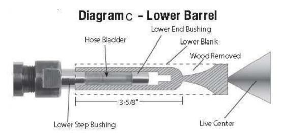
Turning the Lower Barrel see Diagram C
